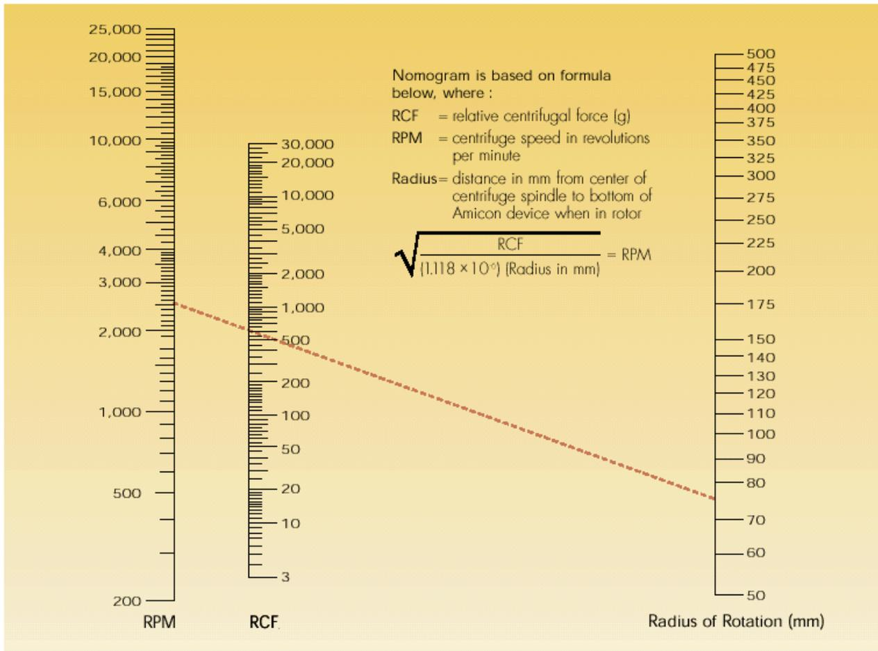
**To convert maximum relative centrifugal force (RCF) to RPM: Determine centrifuge's radius of rotation (in mm) by measuring distance from center of centrifuge spindle to bottom of device when inserted into rotor. Lay a ruler or draw a line from radius value in right-hand column value that corresponds to the device's maximum rated g-force. Then read the maximum value from column at left.**
