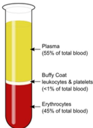
1) Top golden layer = plasma: the plasma layer is usually semi-transparent and golden in color. Transfer **four**, 1mL aliquots of plasma into the two GAPPS supplied and labeled **blue-capped** 2 mL cryo-vials. Avoid the incorporation of the lower buffy coat and erythrocyte layers into the plasma fraction.
